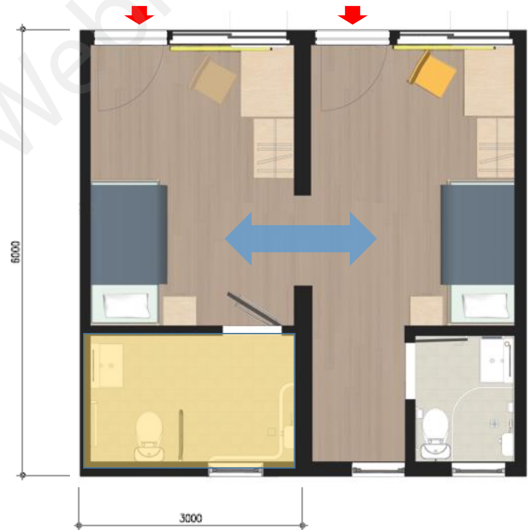
BFA Unit + Companion Unit (2 MiC Modules)
